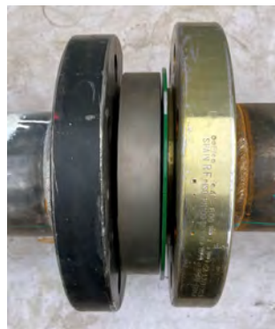
Figure 5 Flanged joint with a High-Performance configuration ring
