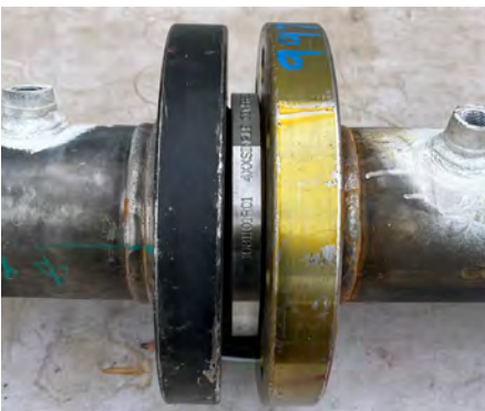
Figure 4 Flanged joint with a standard configuration ring
