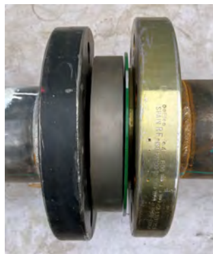
Figure 5 Flanged joint with a High-Performance configuration ring
