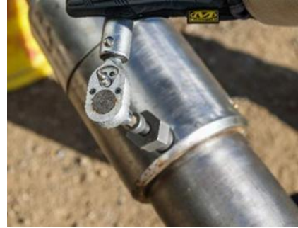
Torque Seal Insert Tool
