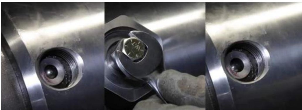
Tightening the bolt to push the ball through the seal
